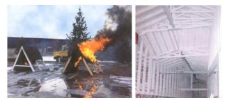
Left: SafeCoat<sup>®</sup> coated interior roof space and an untreated roof space under identical fire conditions. **Right:** According to the NFPA-13 Standard, installation of sprinkler systems are not required if the exposed combustible materials have 25 or less/Class A Flame Spread, re-classifying them as non-combustibles.
