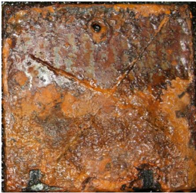
Figure #1: PRECIDIUM™ P-180D Primer no topcoat. This sample was used to evaluate corrosion resistance of P-180D on its own.
