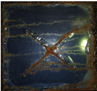
Figure #3: Conventional solvent based epoxy primer and urethane topcoat system. This sample was used as benchmark for a complete primer/topcoat system. The system tested is a widely used commercial system for industrial maintenance applications.
