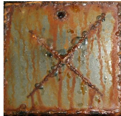
Figure #2: Solvent free two component primer (Standard). This sample was used as a control to determine the corrosion resistance of a P-180D type of product with no anti-corrosion additives employed.
