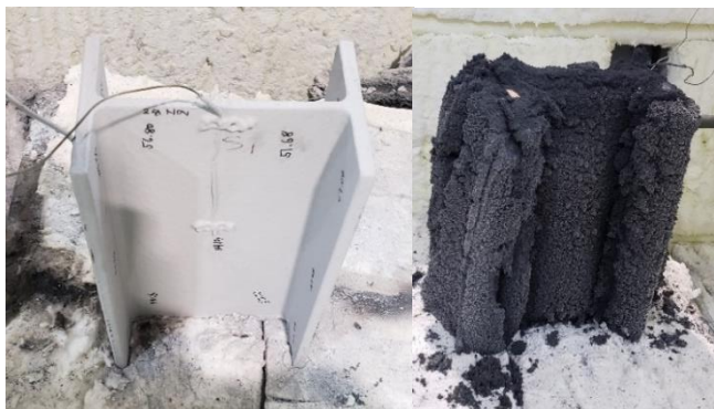
Above: Steel test sample before (left) and after (right) fire test (ASTM E119) showing the thick char that formed and protected the underlying steel
